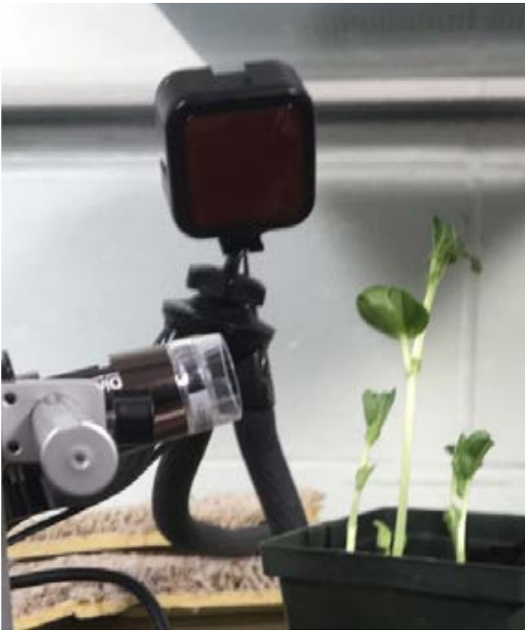
Above: An infrared-sensitive macro camera, and infrared spotlight, center, are used to film individual aphids on a potted plant. Photo by Victoria Salerno.
